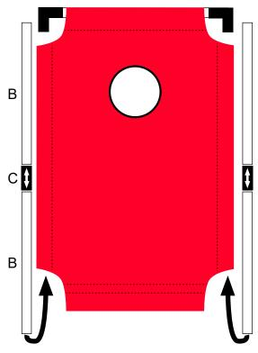
4. Attach Bottom-Tube (A) with L-Shape-Connectors (F)
